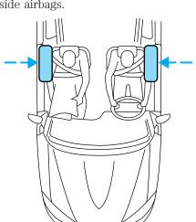
not of the type sufficient to cause activation. Side airbags are designed to inflate in side-impact collisions, not roll-over, rear-impact, frontal or near-frontal collisions, unless the collision causes sufficient lateral deceleration.
